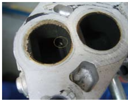
图3 故障车辆上卡滞的EGR阀
